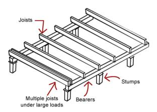
Although it may appear to be a simple structure, it forms the basis of the whole, home or deck. The size of bearer and spans usually needs to be engineered to ensure correct load distribution. If not done correctly, the entire structure can buckle, or worse, collapse.
